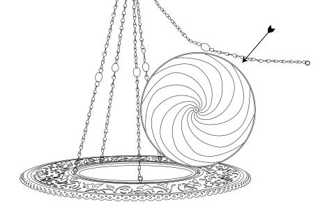
**B.** Insert the lampshade through the chains as shown in the picture.
