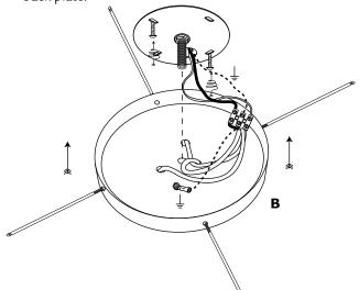
5. Secure the fixture against the mounting surface using the mounting cap C provided//
